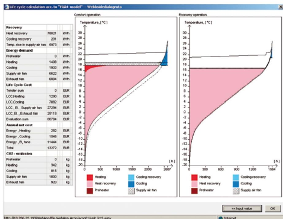
Both the supply air temperature and the exhaust air temperature are supposed to be linear in the degree-hour diagram between the input value for winter and the input value for summer. Calculated heating and cooling capacities account for the heat gain in the fan. When cooling the air to the right temperature and humidity, both the targeted temperature and humidity must be given.
